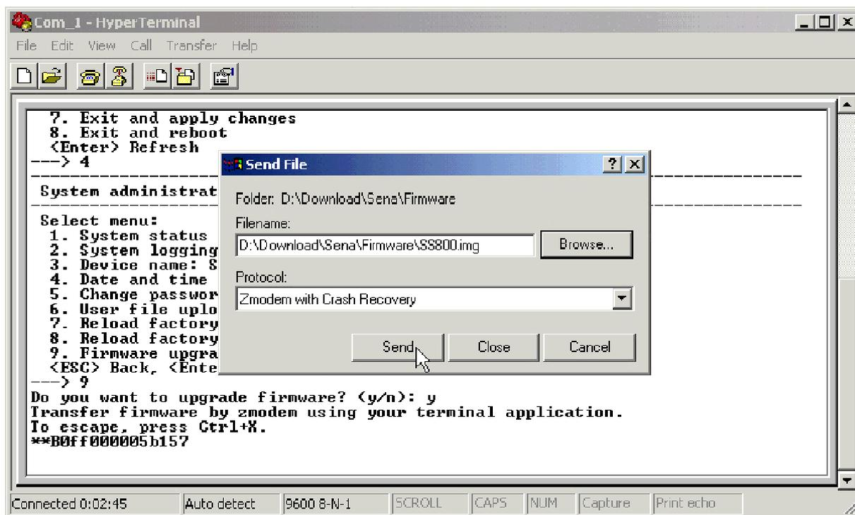
Figure 6-11 Transfer binary file by Zmodem (HyperTerminal)
