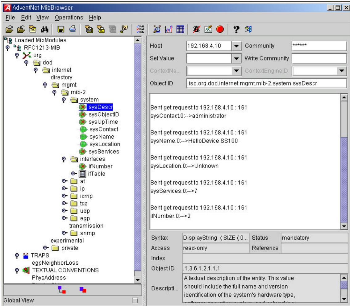
Figure 3-3 Browsing MIB-II OIDs of STS Series SNMP agent using SNMP Browser
