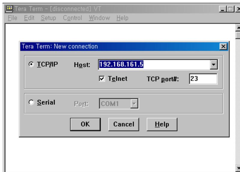
Figure 2-9 Telnet program set up example (TeraTerm Pro)
