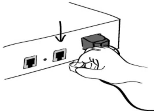
*Figure 2-7 Connecting a system console cable to the STS Series*
