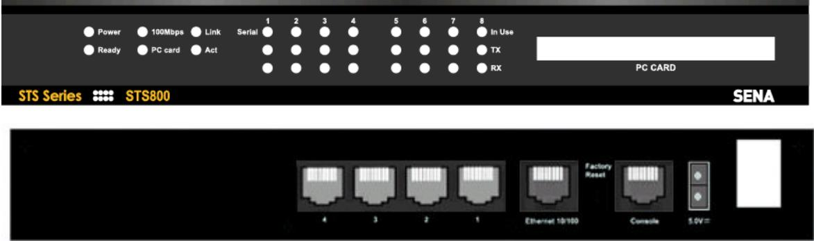
Figure 2-1 The panel layout of the STS800
