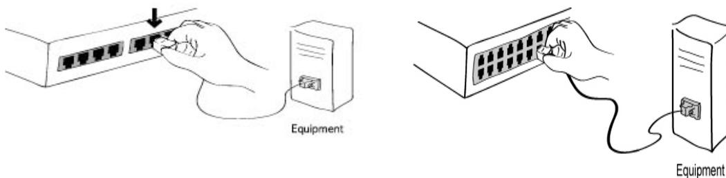
Figure 2-6 Connecting a equipment to the STS400/800(Left) / STS1600(Right)
