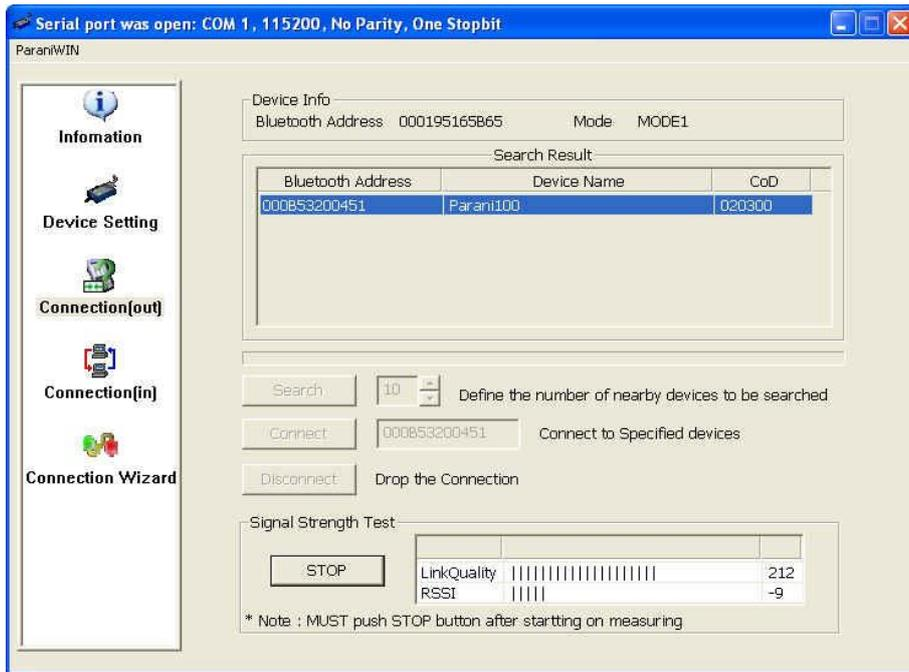
*Figure 3-7 Signal Strength Test*
