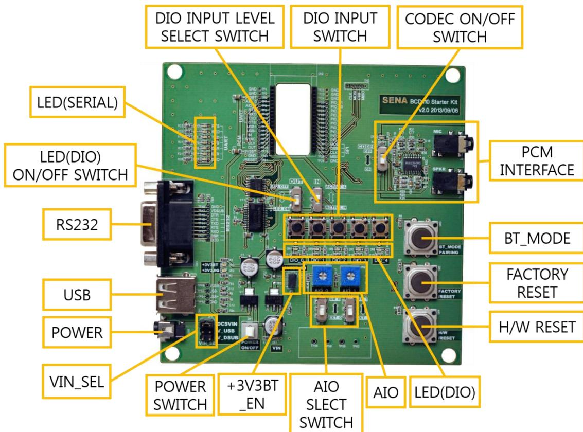
Figure 2-1 The Panel Layout of BCD Development Board
