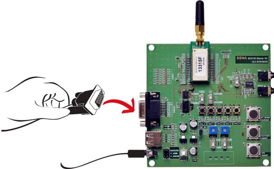
Figure 2-4 Connecting a Device to Development Board
