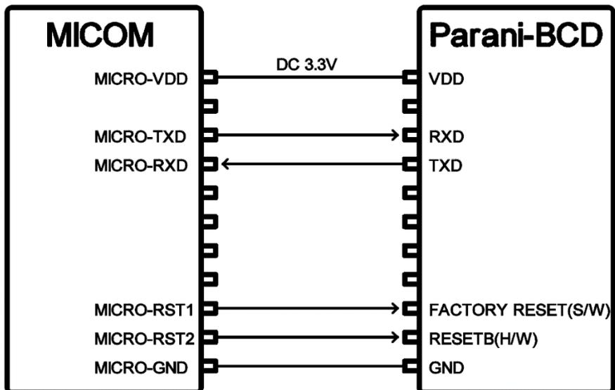
A.2.1.3. When TTL level of MICOM is 5V
