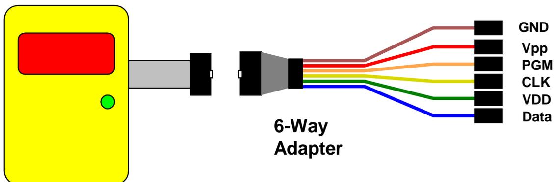
Note: This adapter connects all the GND pins shown in the 10-way connector. If you make your own 10- to 6-way adapter, it should also connect all the GND pins on the programmer lead.
