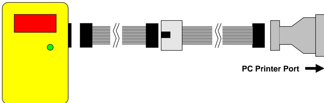
2b) Or, simply connect the PC adapter directly to the programmer using the short ribbon cable.
