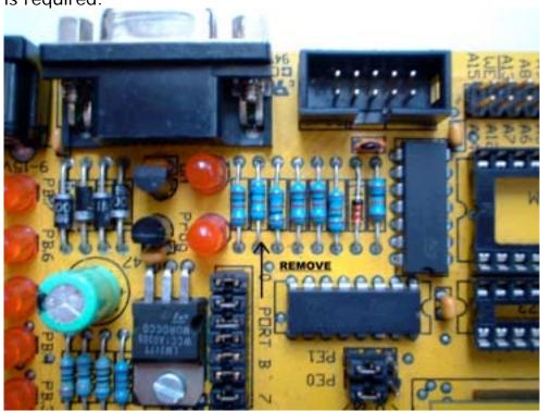
Check the value of the resistor indicated. If the value is 1K, it should be removed. STK200's requires no modification.
