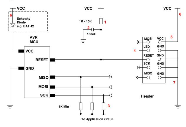
1) This resistor should be fitted. It can larger than 10K if required, but not smaller than 1K
