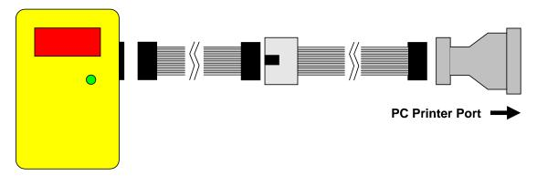
2b) Or, simply connect the PC adapter directly to the programmer using the short ribbon cable.
