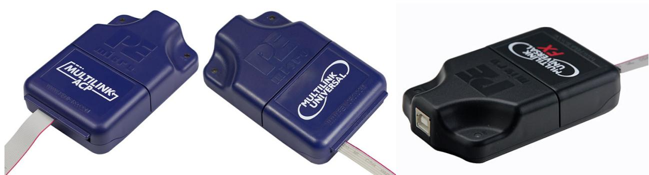
PEmicro's Multilinks allow the user can take advantage of the background debug mode to halt normal processor execution and use a PC to control the processor. The user can then directly control the target's execution, read/write registers and memory values, debug code on the processor, and program internal or external FLASH memory devices. The USB Multilink FX can also provide power to your target MCU, either 3.3V or 5V.
