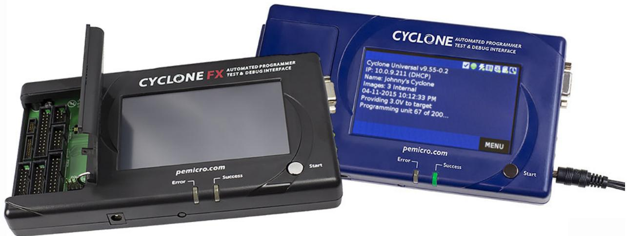
By connecting to a debug header on the target, Cyclone programmers can program internal memory on an ARM Cortex-M processor. SWD/JTAG protocol is used for programming, which requires only 2 pins. The processor or memory device can be mounted on the final printed circuit board before programming.
