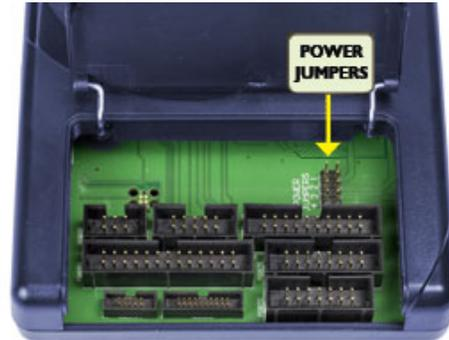
If power is provided via the Cyclone, the user may need to configure the programming image accordingly. Image creation and configuration is discussed in **Section 3 - Creating A Stand-Alone Programming Image**. For more information on the various power configurations, the user should refer to their Cyclone's User Manual. There is also a blog post that covers this topic at: [http://www.pemicro.com/blog/index.cfm?post\\_id=121](http://www.pemicro.com/blog/index.cfm?post_id=121)
