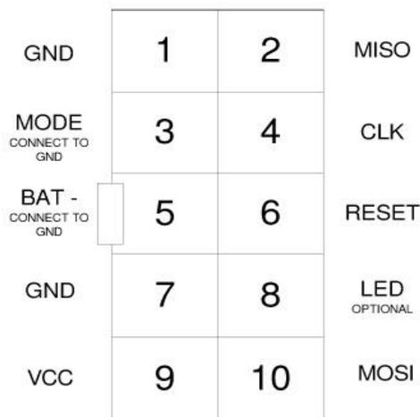
TOP VIEW OF THE CONNECTOR ON
