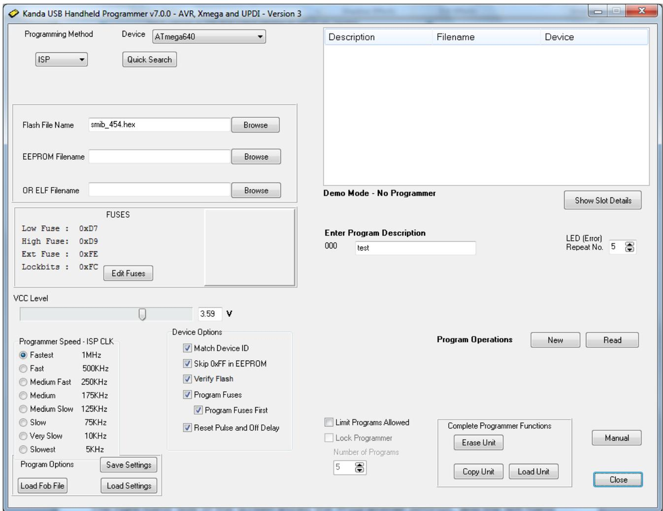
The right-hand side of the screen shows the Programmer settings, and the left-hand side shows details about the AVR (or ATxmega) device, filename, programming method, fuses and other details that will be used to load the programmer. This is single programmer screen, 8-way programmer adds some buttons (Delete and Replace).
