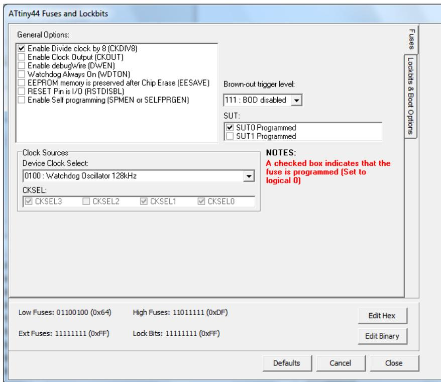
The available fuses and lock bits for the currently selected AVR are displayed. Click on the tab on the right of the screen to **see Lockbits and Boot Block** options.
