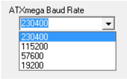
You will also need to slow down baud rate for lower voltage applications e.g. 57,600 at 1.9V.
