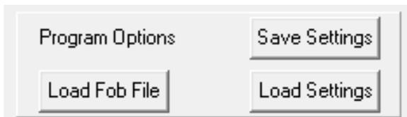
Located at button left of the screen, the **Load Fob File** button allows all the settings to be updated from a Fob file (.fob) that has been saved from earlier versions of AVR Handheld software.
