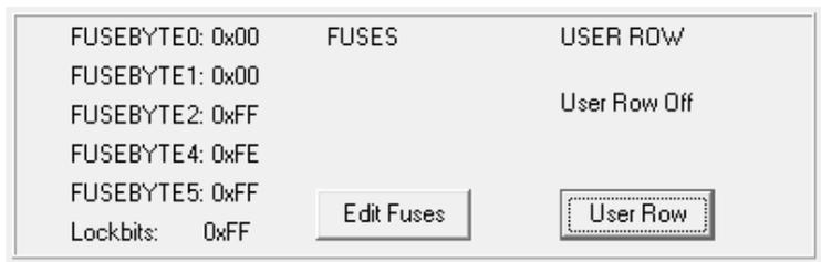
There are 5 Fuse bytes but Fuse byte0 is JTAGID and only available if device has JTAG Interface. Edit Fuses button works the same as AVR section.
