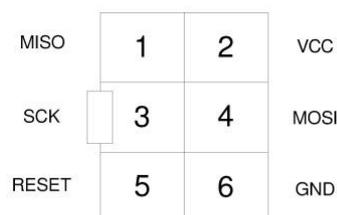
TOP VIEW OF THE CONNECTOR ON
