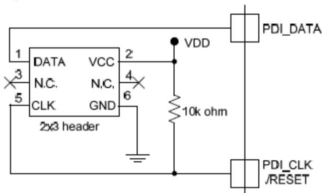
PDI programming default speed is 230,400 baud so any capacitance on programming lines will create problems. Slow it down if you get 2 red error flashes.
