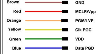
For Low Voltage programming, connect 6-way adapter directly to key fob programmer. For High Voltage Programming, insert 12V generator board between keyfob and adapter as shown below.
