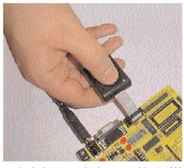
car key fob type so it is easy to source and we even include a spare in the starter kit. A 12V generator for High Voltage programming and an adapter for converting the 10-way connector to 6 Flying leads come with the programmer.
