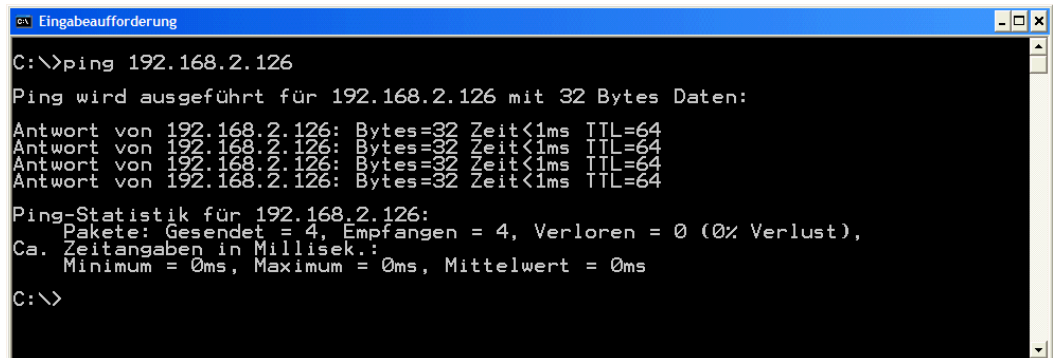
Figure 25: Checking the new IP address with ping
