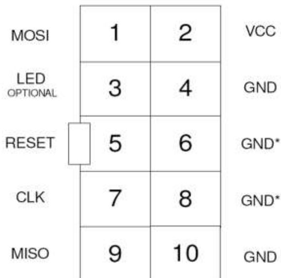
TARGET CONNECTOR FOR AVR PROGRAMMERS
